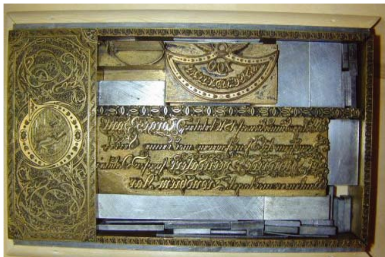
Above: The first banknote type. One speciedaler, signed 1822. Right: Print plate for the 100 speciedaler note. The larger denominations had the same format (123 x 190 mm), the 1- and 5-speciedaler notes were slightly smaller, and the 1/2- and 1/5-notes about half the size
